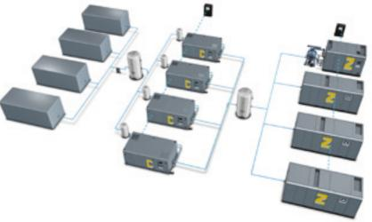
Machines of different sizes managed with ES controllers, delivering air to Strech Blow Moulding machine for PET bottle production
